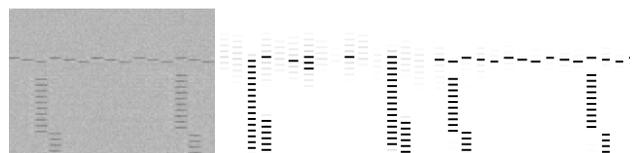
**Figure 19.** Zoomed examples of droplet detection: input image (left); without correction mask (middle); with correction mask (right)
