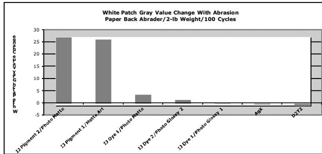
**Figure 2: Relative sensitivity of photographic printer/papers to abrasion.**
