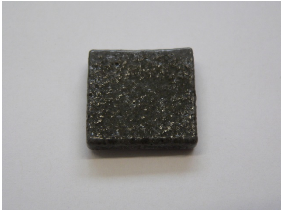
Figure 6. Efflorescence glazed 3D printed tile
