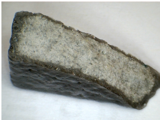
Figure 7. Section showing glaze surface
