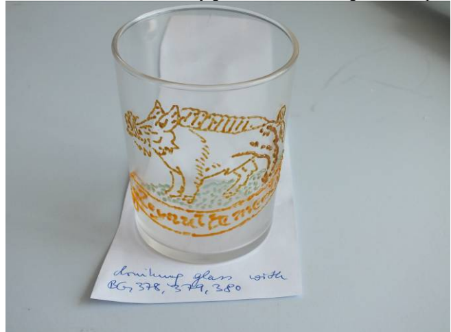
Figure 3: Embellishment printed on a glass. Only a single layer was applied. The printing time for the 3 colour print was about 10 min.
