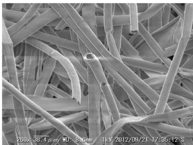
Figure 11 SEM image of paper sheet made from only Kapok fibers.
