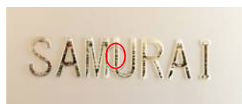
(a) Sample with poor quality based on bad leveling UV primer ink.
