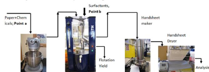
Figure 1: Schematic of Deinking Study.
