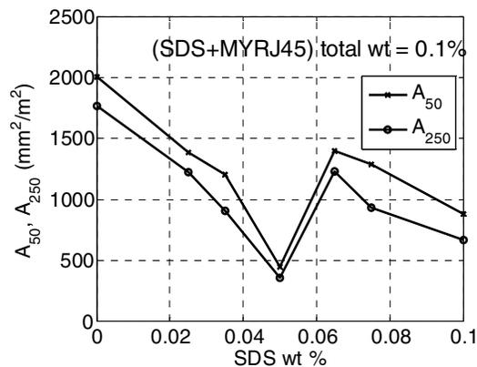
Figure 5: A blend of nonionic surfactant (MYRJ 45) and anionic surfactant (SDS) is added during flotation. The chemistry of pulping was HPMF. Total weight of surfactant was kept at 0.1 wt%. This at the point where SDS wt% is 0, MYRJ 45 wt% is 0.1.
