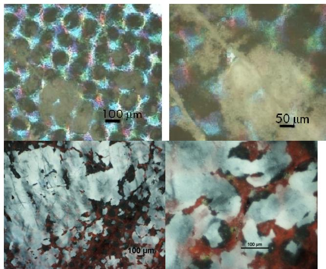
Figure 3: Ink specs seen in HPMF deinking; paper #1 is shown in the top two optical micrographs and paper #8 is shown in bottom two optical micrographs.
