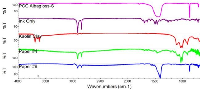
Figure 4: FTIR measurement of ink specks from paper #1 and paper #8 are shown. FTIR of PCC, clay and LEP ink are also shown.
