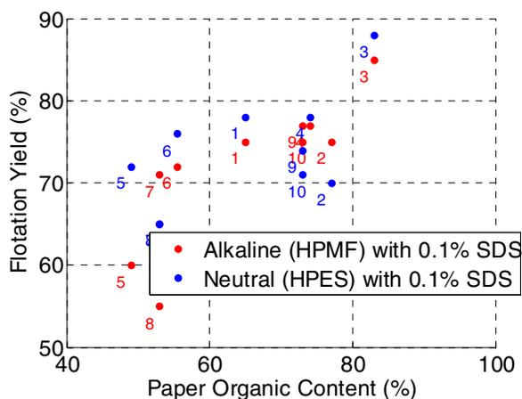
Figure 2: Flotation Yield vs. Paper organic content. Paper organic content is measured by TGA in air atmosphere. The numbers inside the figure represent paper numbers.
