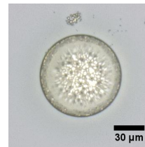
Figure 8. Via in top view after the deposition of 32 drop in 16 fractions of 2 drops with a waiting time of 60 s. Substrate temperature 80 ^{\circ}\text{C} . Depth of field from wafer surface to via bottom.
