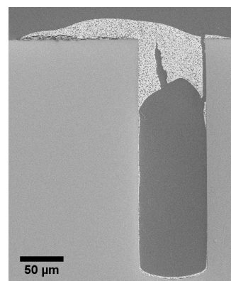
Figure 3. SEM cross sectional image of a via after sintering at 300 ^{\circ}\text{C} for 30 min. 120 drops deposited with a waiting time of 15 s and a substrate temperature of 70 ^{\circ}\text{C} .
