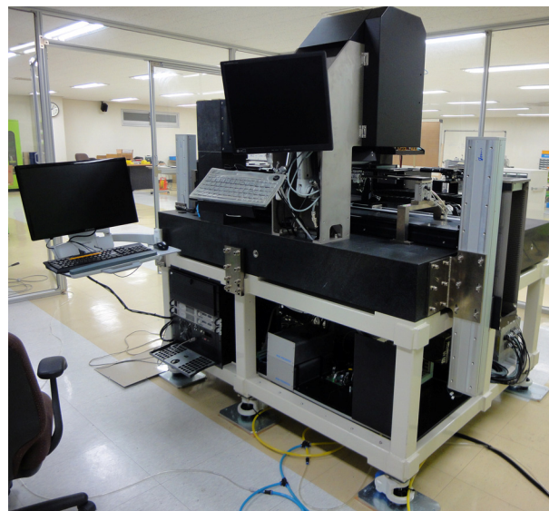
Figure 1. Developed ink-jet printer, SSP-01, for the front side metallization of a solar cell wafer.
