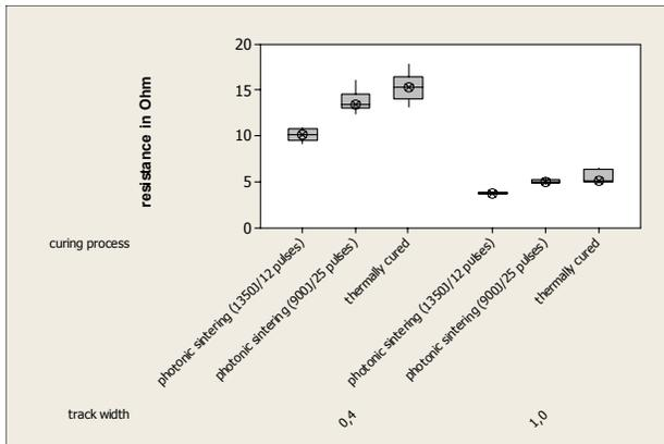
Figure 5. Initial resistance values of conductor tracks on FR-2 after photonic sintering with two different energy levels for both track widths (reference values: thermal curing 180°C/1h)
