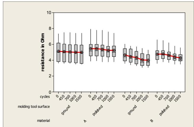
Figure 4. Effect of thermal cycling on the resistance values of conductor tracks (width 1mm)
