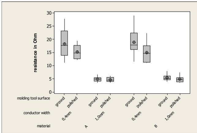
Figure 3. Initial resistance values of conductor tracks
