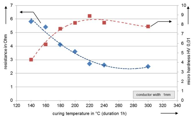
Figure 2. Development of resistance and micro hardness as a result of curing conditions
