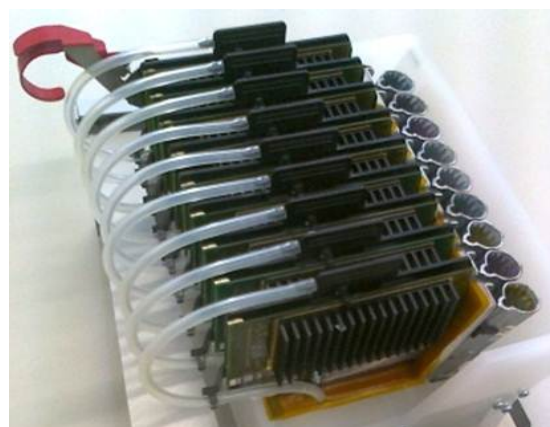
Figure 2, Print head array with 9 CrystalPoint print heads as used in the PiXDRO JETx.
