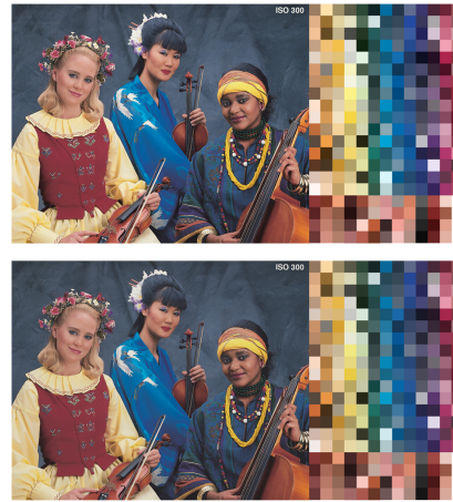
Figure 2 An example of the printed test image pair (N7) with its 256 typical color patches
