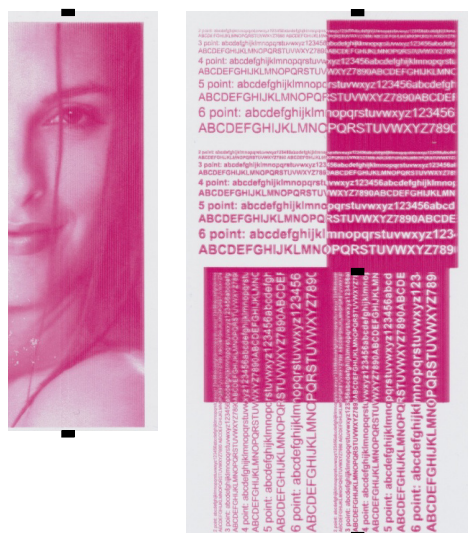
Figure 6. Print samples in which the volume control method has been used to stitch print swatches.
