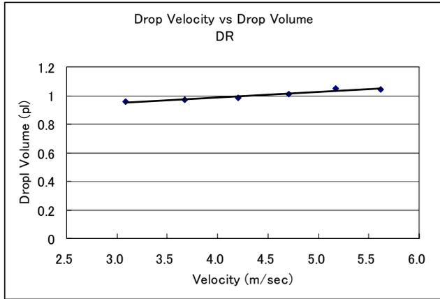
Fig.8 Drop Velocity vs Drop Volume
