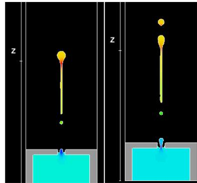
a) Satellite-free condition b) With satellite condition
