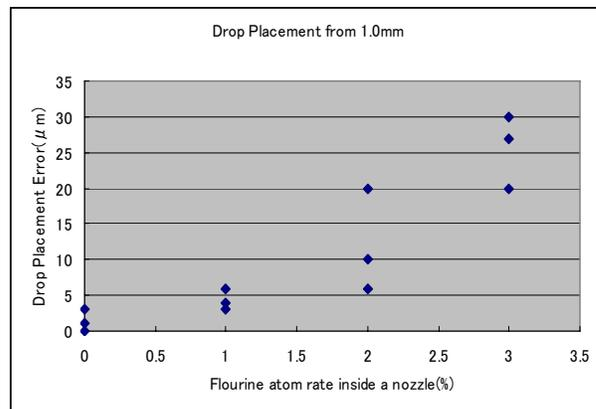
Fig.6 Drop Placement Error vs Non wet layer Processing accuracy
