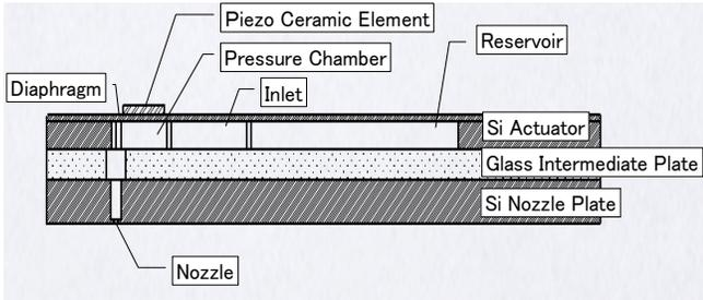
Fig.2 Cross section of an individual MEMS head
