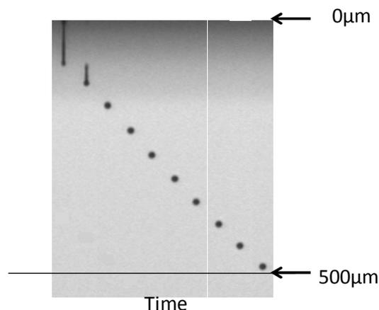
Fig.7 Transition of filament shape at satellite free
