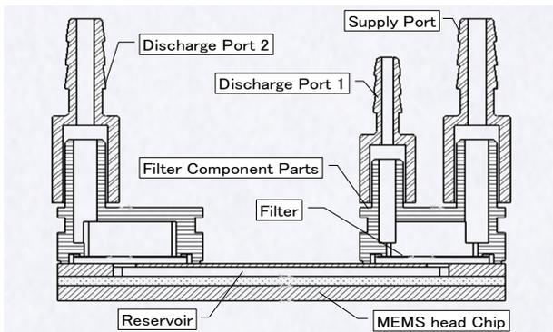
Fig.3 Cross section of MEMS head chip & Ink supply
