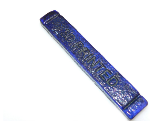
Figure 7. 3D printed test bars with efflorescent glaze
