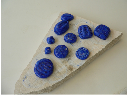
Figure 5. Egyptian Faience test body
