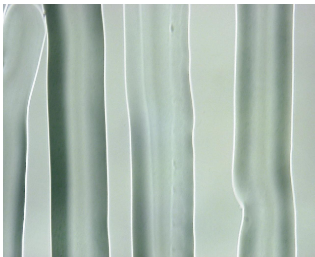
Figure 4 Line structure of calcium alginate utilizing the PELID method.
