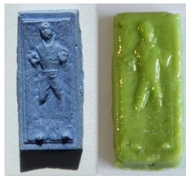
Figure 5: On the left, the sample is made from particles with an average diameter of 700 nm. On the right, the average particle size was 50 \mu\text{m} . Both samples were fired following the same firing schedule.
