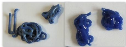
Figure 3: For glass sample on the left 40wt% of saccharides were used as binder, for the one on the right only 5wt%. The left one is discoloured, the right one not.
