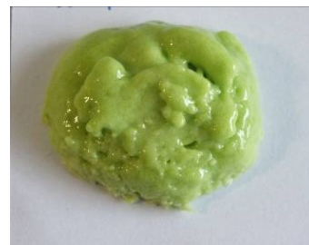
Figure 1: Glass sample with sodium silicate solution as the index matching fluid. Firing of the sample leads to bubbling and loss of all detail.
