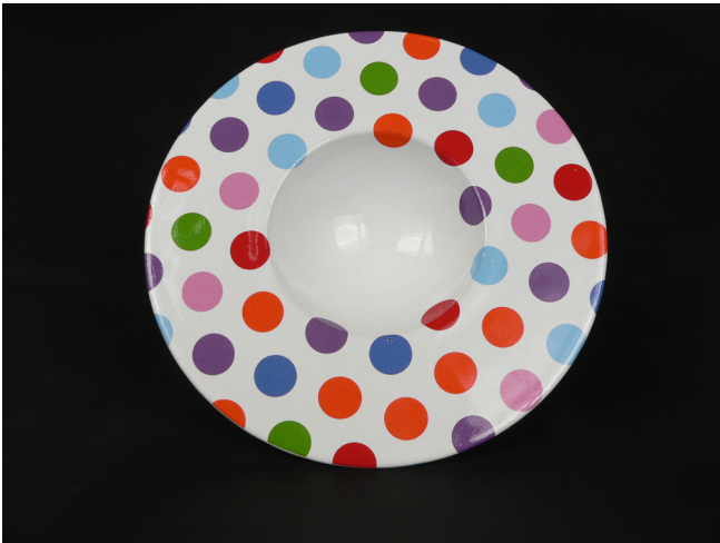
Figure 8. Glazed decorated 3D printed ceramic
