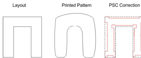
Figure 15. Layout, Printed Pattern and PSC Correction for U-shaped structure
