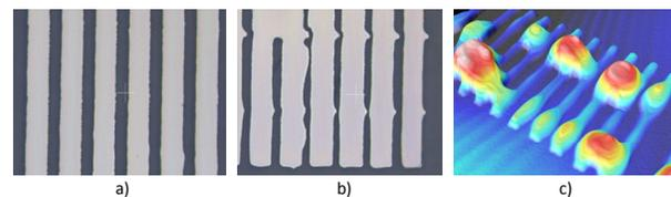
Figure 12. a) Correct spacing, b) Printer misalignment, c) Electrical shorts
