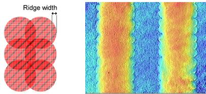
Figure 7. Ridge width effect of scalloped lines
