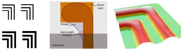
Figure 14. Designed, printed and 3D image of corner patterns
