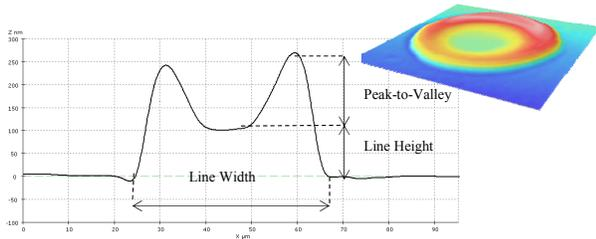
Figure 3. 3D and sectional image of a drop and bead parameters defined.
