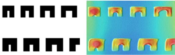
Figure 13. Test pattern and 3D image for minimum notch rule extraction
