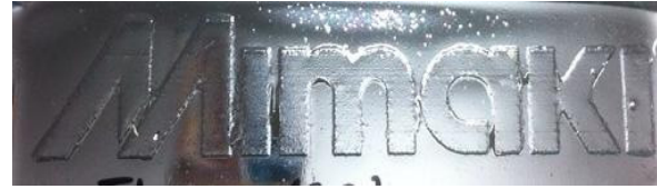
Figure 3. Print sample by Digital quasi-embossing technology
