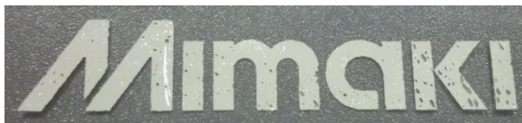
Figure 5. Print sample by digital quasi-embossing technology for partial transfer of metallic layer
