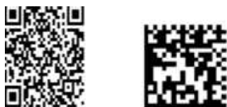
Figure 4. Example of two different 2D bar codes. On the left is a QR Code bar code, and on the right is a Data Matrix bar code.
