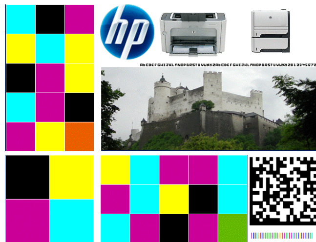
Figure 3. Print-print hybrid packaging. The original size of the “medallion” is approximately 1.5 x 1.0 cm. The colored tiles in the upper left and lower center can be read by mobile cameras, while the tiles in the lower left are used for color calibration. A 2D bar code and set of color bars are in the lower right. In the center and right center, the image of the castle contains a digital watermark. At the top center and right, the brand mark and product pictures are used for product identification. Beneath these images there is variable-data printed microtext, which is not readable after copying.
