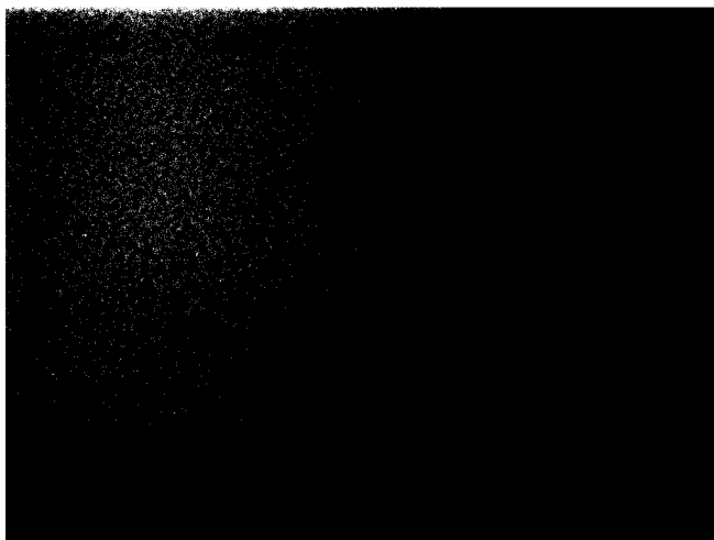
Figure 9: Light field measurement of CCD array, light normal to array surface. White points indicate pixels with readings in the top 10% of all measurements after dark field calibration.
