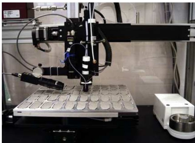
Figure 2. Precision printing of explosive compounds on substrates for the testing of trace detectors.
