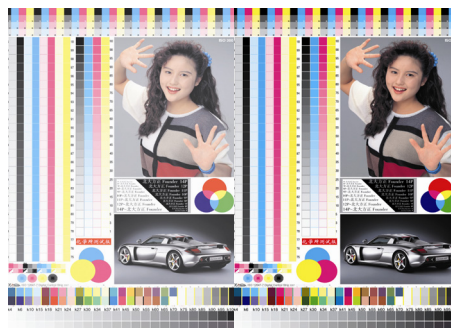
Fig. 3 Print samples produced by printing plates with different roughness; Left: the plate with proper surface roughness; Right: the plate with wrong surface roughness.
