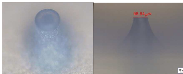
Figure 4. Oblique view of glass nozzle (left) and side view of the nozzle (right)
