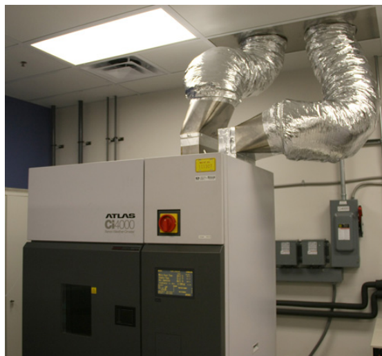
Figure 1. Atlas Ci4000 Weather-Ometer with air intake modified to bring in unfiltered air from the building rather than using filtered lab air.
