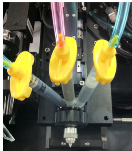
Figure 2. nScript 3 material micromix dispensing tool
