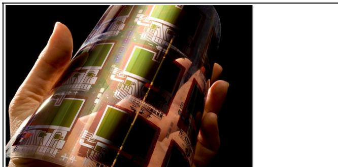
Figure 1: 6" by 6" flexible solar cell modules on foil.
