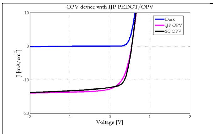
Figure 7. Device performance of OPV devices with benchmark of spin-coated and inkjet printed PEDOT:PSS and inkjet printed PAL layers.
