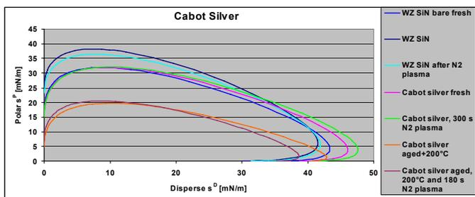
Figure 5: Measured surface energy of WZ SiN and Cabot silver ink.
