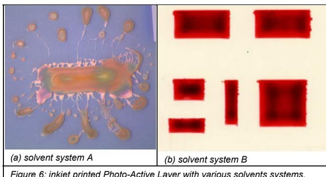
Figure 6: inkjet printed Photo-Active Layer with various solvent systems.
