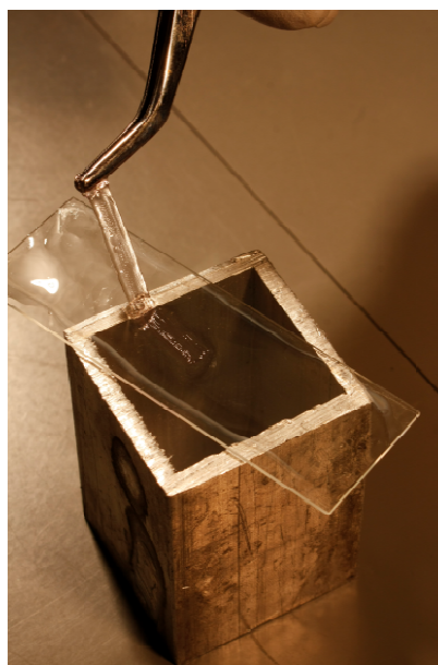
Figure 2. Printed hydrogel (10% MA and 10% gelatin, both solutions in 0.1M borax) using a modified HP Deskjet 340 Printer.
