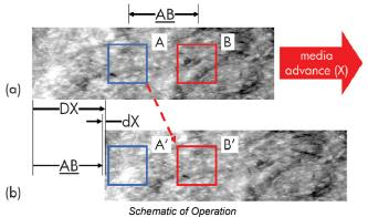
(a) media at first position (b) moved a distance DX in the X-direction
