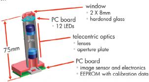
Details of Optical Media Advance Sensor - Sensor Module
