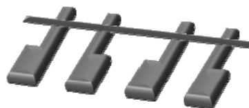
Figure 3. Schematic representation of the printed template with four silver electrodes/antennae and a single silver line inkjet printed on top of the antennae. The total length of the line is 1.6 cm.
