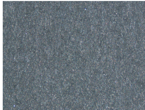
Figure 2: Surface scan of desirable roller under 200X magnification. No microscopic bubble is observed.
