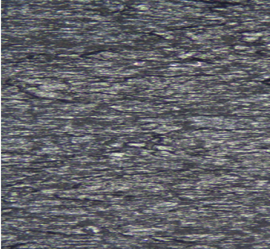
Figure 4: Magnified surface texture of questionable roll which can cause bad print quality.
