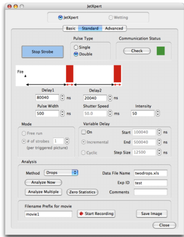
Figure 1: JetXpert strobe control user interface (GUI): Standard Tab showing a double pulse set-up
