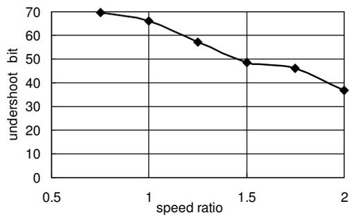
(d) Effect of speed ratio (sleeve speed to drum speed)
