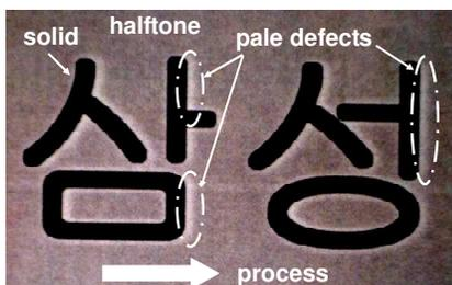
Fig. 1 Example of pale image defect observed in halftone area immediately after printing of solid image.
