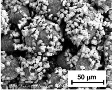
Fig. 3 SEM image of mixture of toner (6  $\mu\text{m}$ ) and carrier (40  $\mu\text{m}$ ) particles (toner/carrier concentration, 6 wt%).
