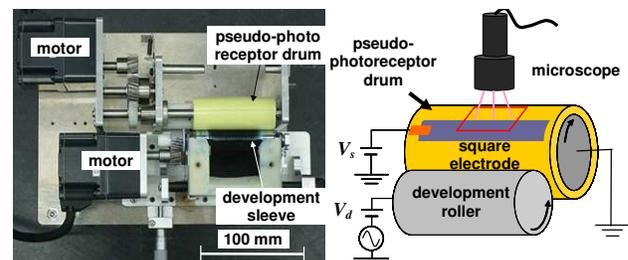
Fig. 2 Apparatus used to model a two-component magnetic brush development system.
