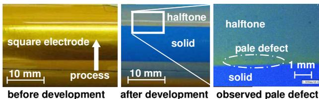
Fig. 4 Surface of the pseudo-photoreceptor drum before development (left) and after development (middle), and end edge of solid image after development (right).
