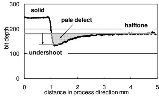
Fig. 5 Circumferential distribution of blue bits at the boundary between the trailing edge of the solid image and the halftone image.
