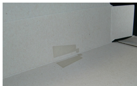
Figure 5: Printed 3D antenna on a folded / erected cardboard box
