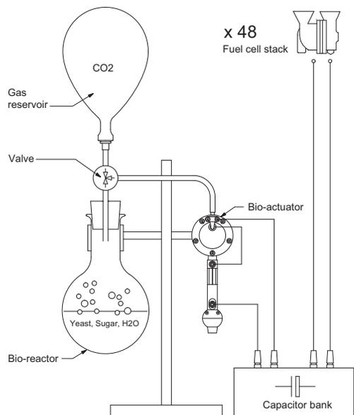
Figure 7. Bio-actuation experiment
