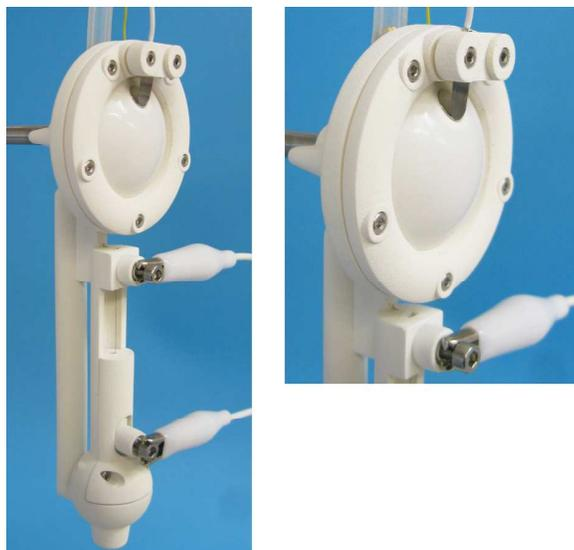
Figure 3. Bio-actuator 3D printed working prototype.
