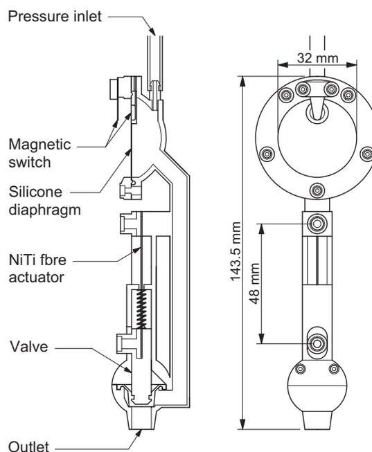
Figure 2. Bio-actuator design.
