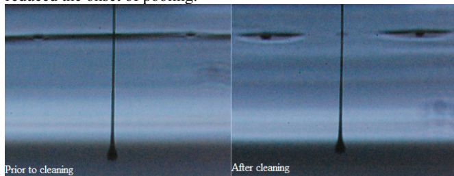
Figure 8. Pooling around non-firing nozzles when printing at 1dpd. When observed after prolonged initial printing the pools were slower to form (left) than when the nozzle plate was cleaned with solvent immediately prior to observation (right). The same effect of delaying pool formation was observed when the nozzle plate was wiped in concentrated surfactant solution.
