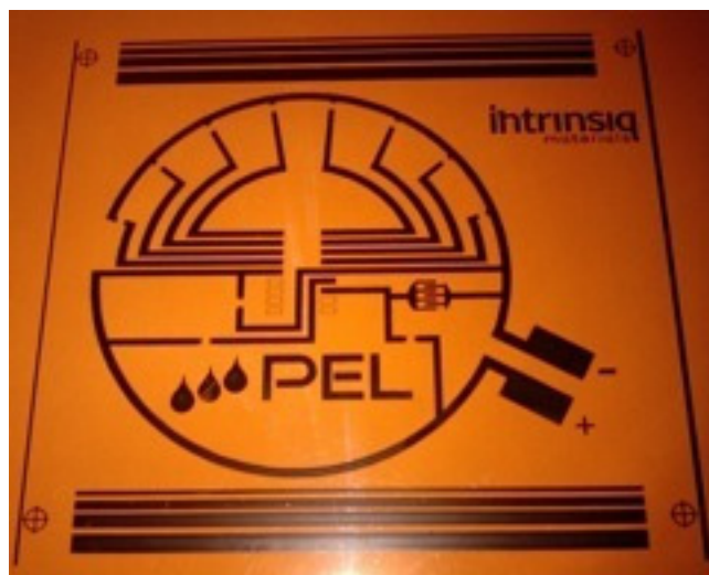
Figure 4. Print of copper ink on various Kapton
