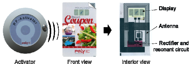
Figure 1 A radio activated display based on a radio frequency rectifier and an electrochromic display. The display information is revealed when being activated in the electromagnetic field of the activator unit.
