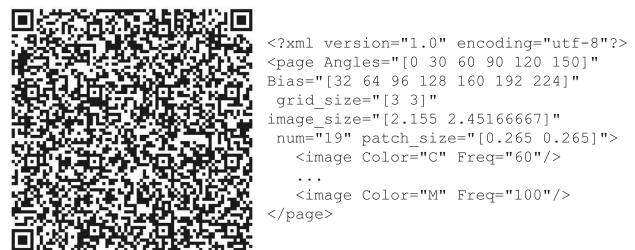
Figure 2. A sample QR code describing a test page, and the embedded XML description.
