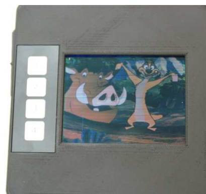
Figure 7. Picture of the full color single layer ChLCD panel showing a color graphic image.
