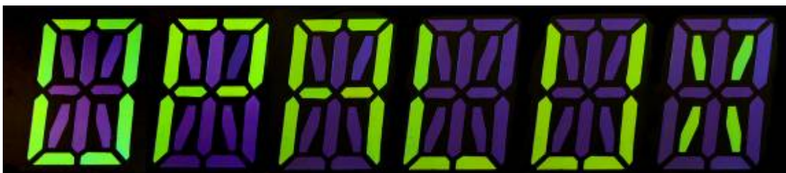
Fig. 4: A pixilated alphanumeric P-Ink display device spells "OPALUX" under ambient office lighting
