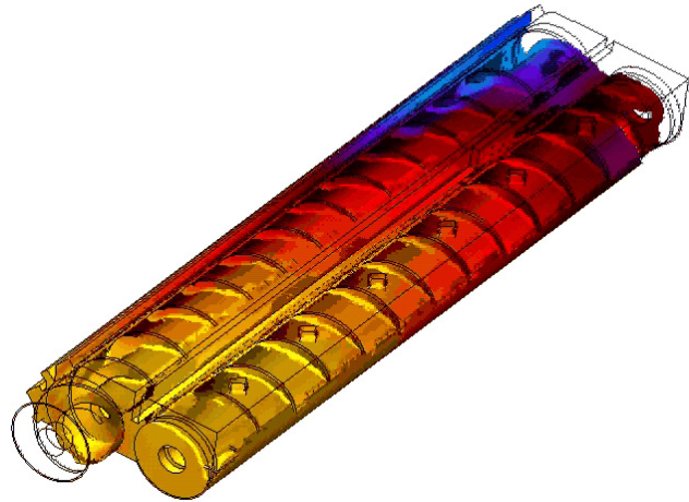
Figure 6. Continuum Model Results of Auger Mixing- Concentration of New Toner
