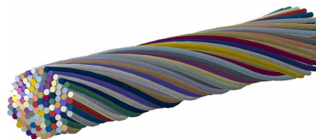
Figure 2. Geometry of a FEM construction of a yarn in textile.
