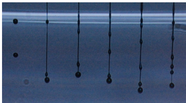
Figure 1 Droplet ejection showing the drop formation of a single cycle greyscale shared wall Xaar 1001 actuator
