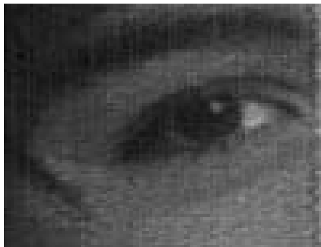
Figure 4 Close up view of a monochrome image printed at 1.27 \text{ ms}^{-1} using the Type 3 head
