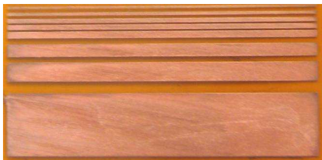
Figure 9. Demonstrator test pattern (Cu plated on PI) created by the catalyst-layer approach.
