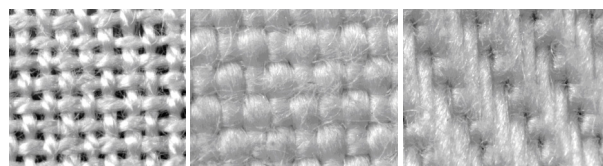
Figure 1. Open and closed plain-woven fabric and a closed 3-1 twill fabric.
