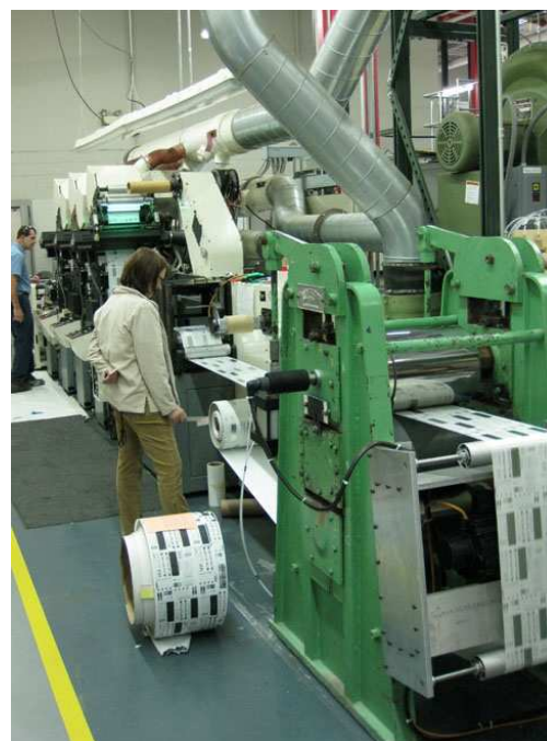
Figure 3. In-line set-up of calendering unit built and placed at the end of a flexographic printing press.
