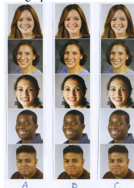
Figure 13: Printed samples presented for survey. Row A was printed at 133 lpi by Heidelberg Speedmaster CD 74 press. Row B was printed by Kodak Prosper press. Row C was printed at 150 lpi by Heidelberg Speedmaster CD 74 press.
