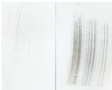
Figure 12: Ink marks scratched off from solids printed by Heidelberg Speedmaster CD 74 press (left) and Kodak Prosper press (right).
