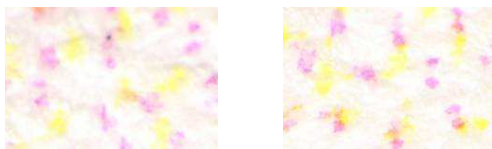
Figure 11. Microscopy images of a 10% red surface printed out on paper with a low (left) and high (right) amount of surface fixation.
